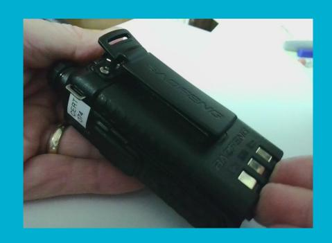
The battery should be flush with the case bottom.
