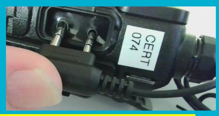
Make sure the radio is powered off before installing earbud
