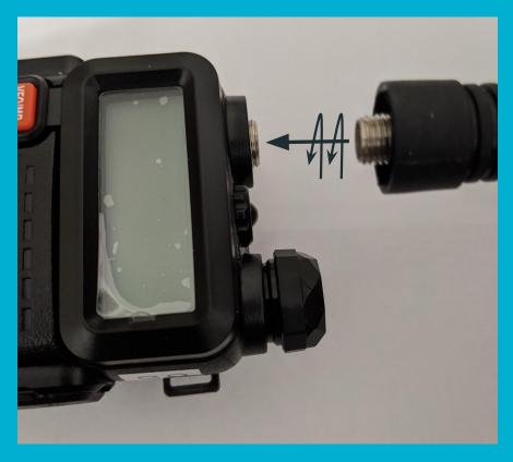
Screw antenna into Radio top.
